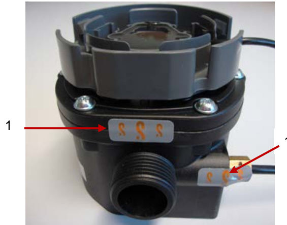
Seals installed in the factory (1) on flow meter and temperature sensor of the Superstatic 789
